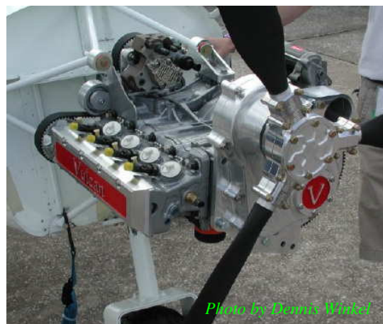
Vulcan Aircraft's prototype Raptor 105 turbo diesel engine
