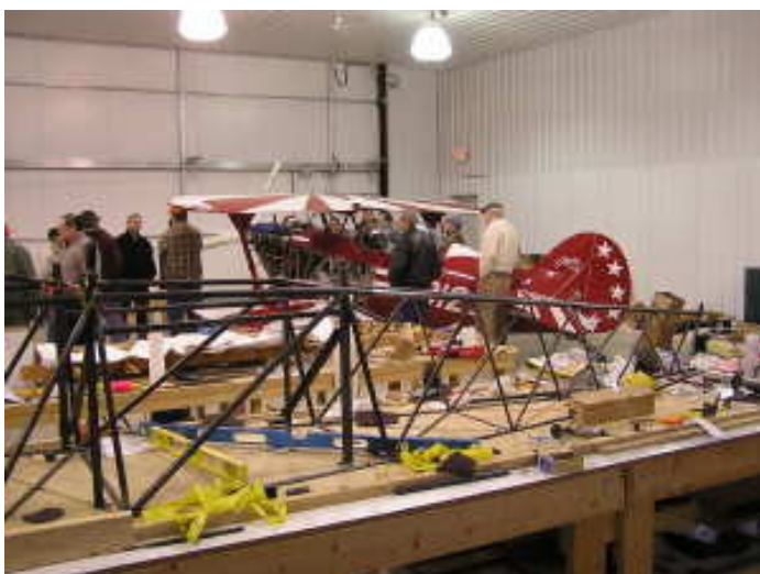
Craig Henry is also building a Pitts Little Stinker. Tack welded Fuselage seen here.
