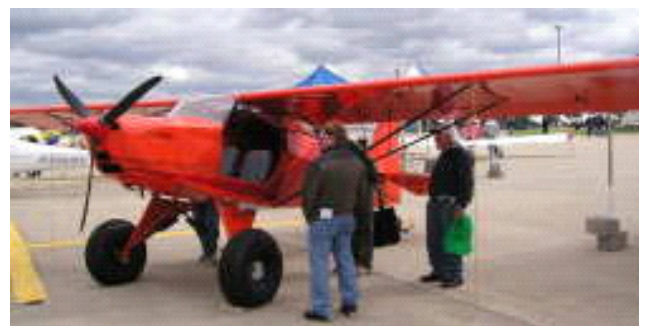
Highlander by JustAircraft powered by a Rotax 912-S 100hp
