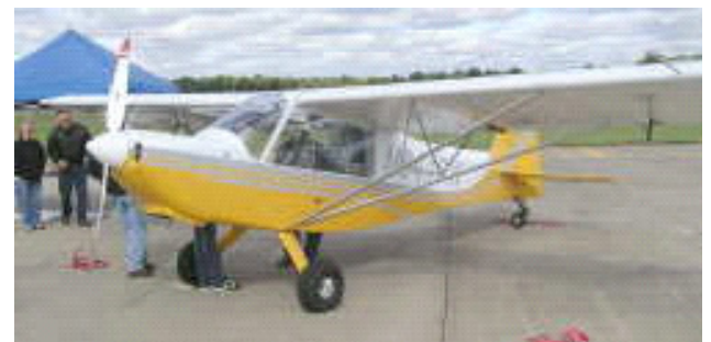
Rans S-7LS powered by a Rotax 912ULS 100hp
