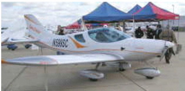
Sport Cruiser RTF powered by a Rotax 912-S 100hp
