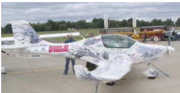
FA-04 Peregrine powered by a Rotax 912ULS 100hp
