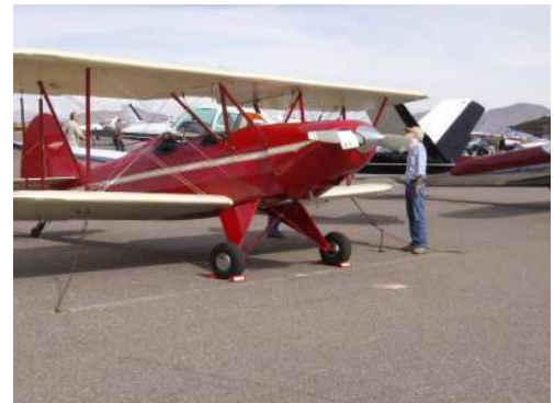
Martin Schmunk's Hatz Special from Fountain Hills, AZ Powered by a Lycoming O-235
