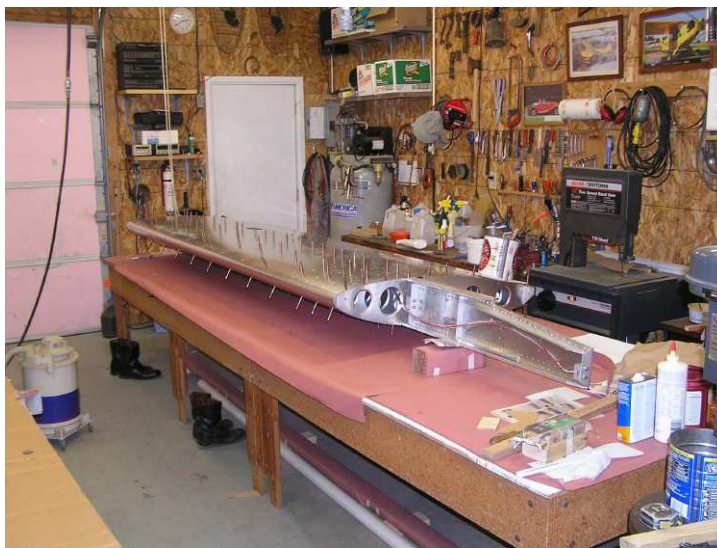
Left wing being skinned. By now the right wing is skinned
